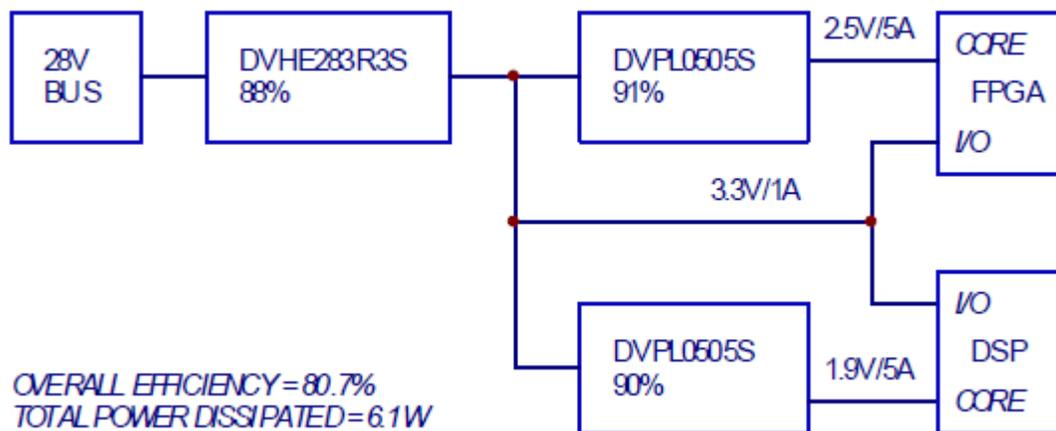
Figure 5. Low Voltage Application Using the HERO Power System.
