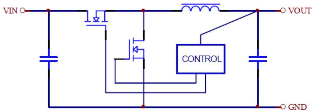
Figure 4. Non-Isolated Synchronous Buck Schematic.
