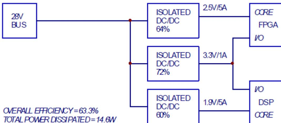
Figure 1. Low Voltage Application Using Isolated DC-DC Converters.
