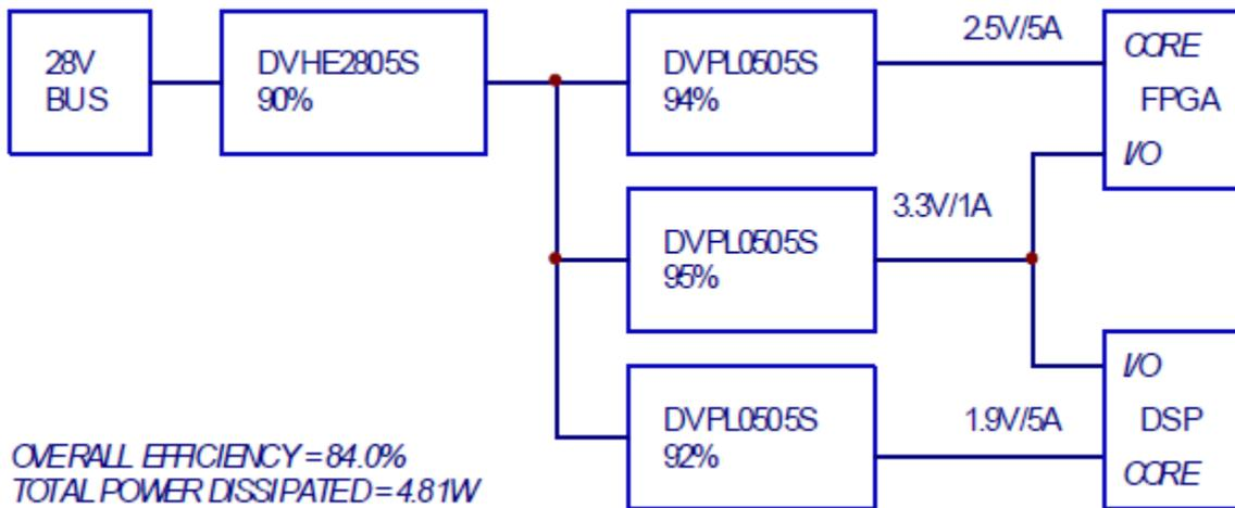
Figure 6. Low Voltage Application Using the HERO Power System Distributed 5V Bus Approach.
