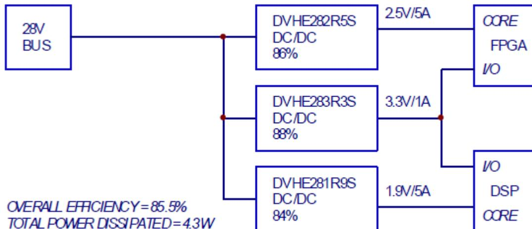
Figure 2. Low Voltage Application Using the DVHE2800S Series.
