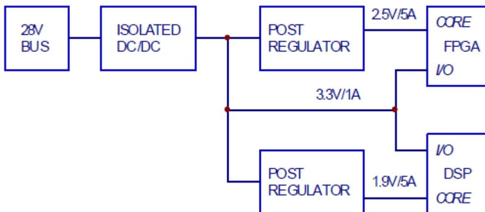
Figure 3. Low Voltage Application Using Post Regulators.
