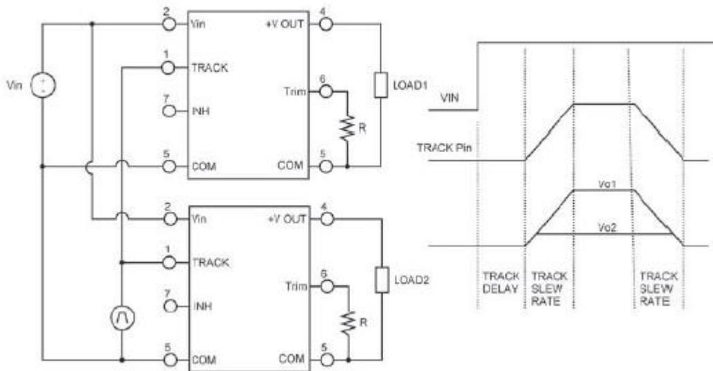
Figure 3. Tracking waveforms.
