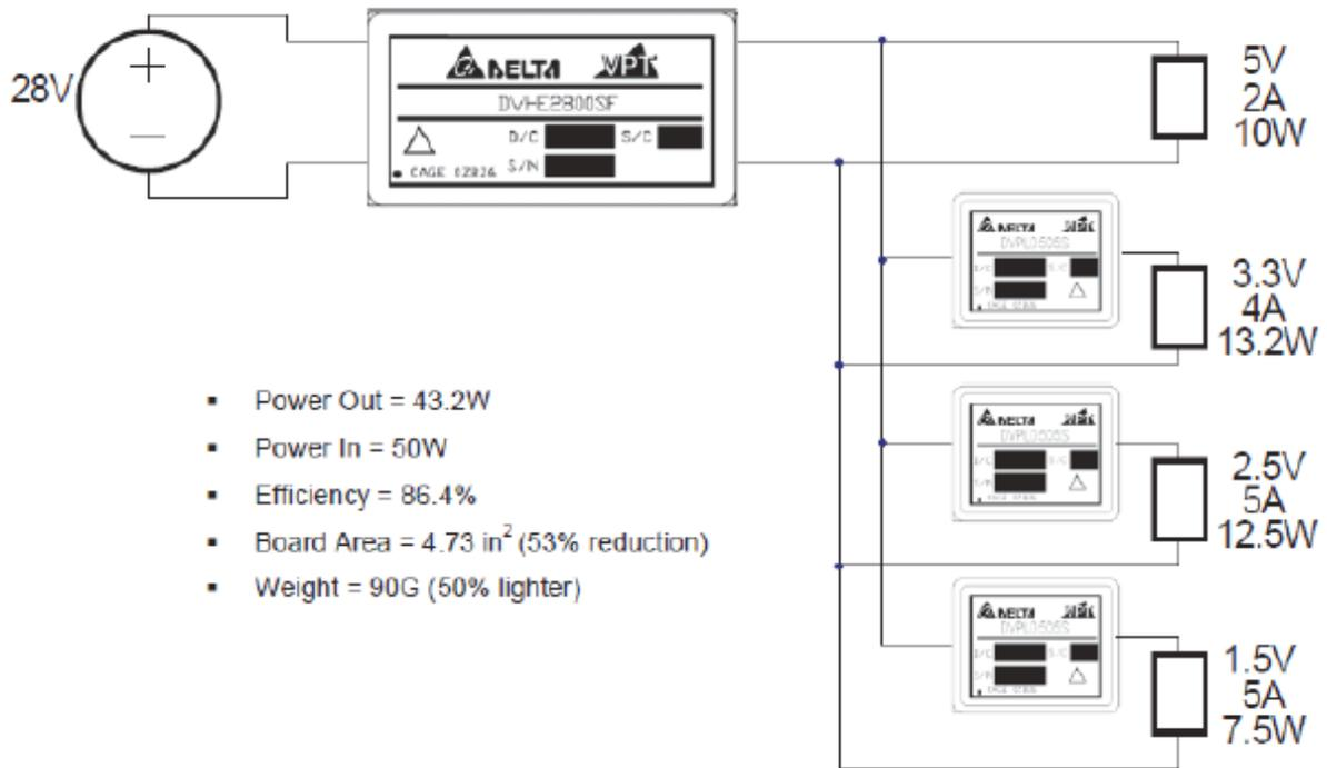
Figure 2. Point of load system approach
