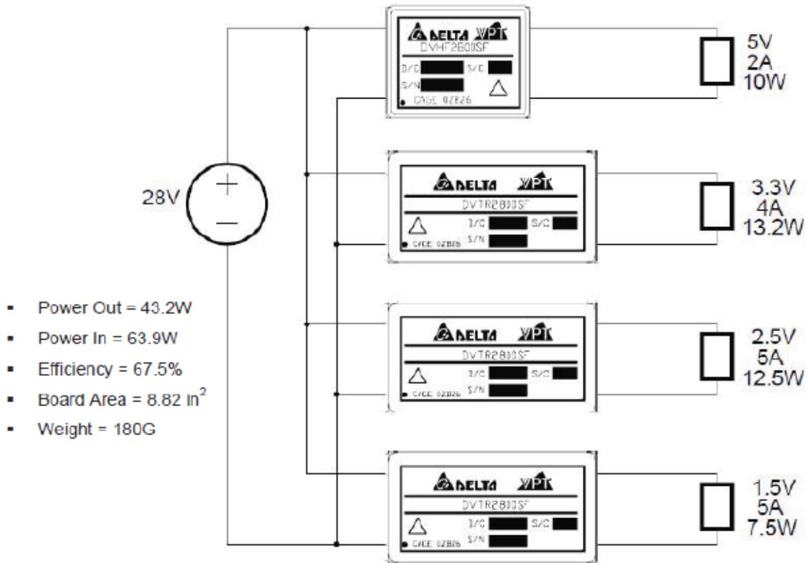
Figure 1. Traditional power system using isolated DC-DC converters.
