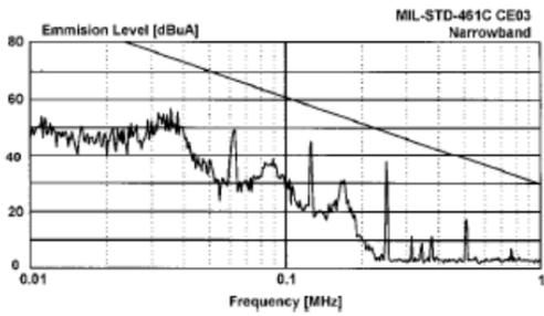
Figure 3. MIL-STD-461C DV200-2812D with DVMN28 EMI Filter.
