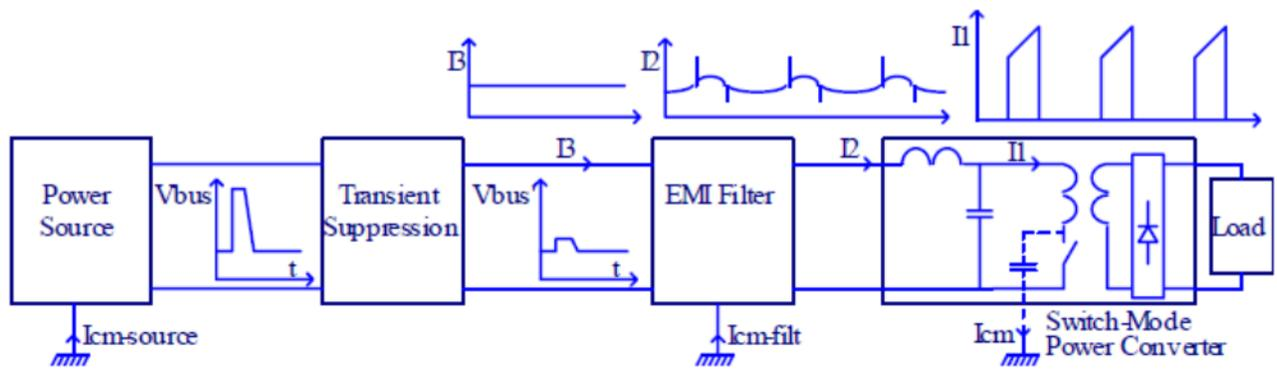
Figure 1. Effect of the EMI Filter and Transient Suppression Functions.
