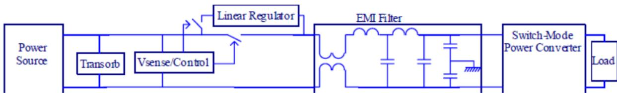
Figure 2. Transient Protection and EMI Filter Discrete Solution Block Diagram.
