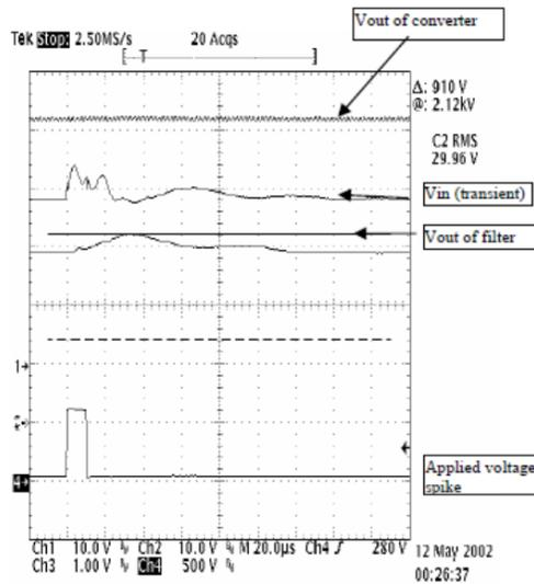
Figure 4. Transient Performance of a Packaged DVMN28 EMI Filter/Transient Suppression Module with DV200-2812D Converter.
