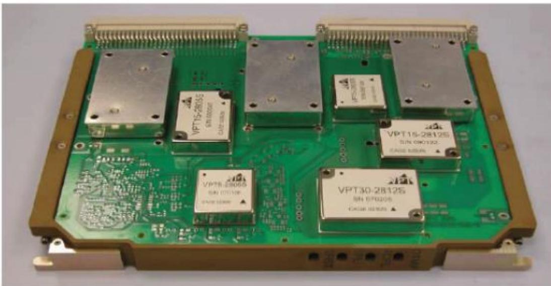
Figure 6. VME power supply built from off-the-shelf DC-DC converter modules.
